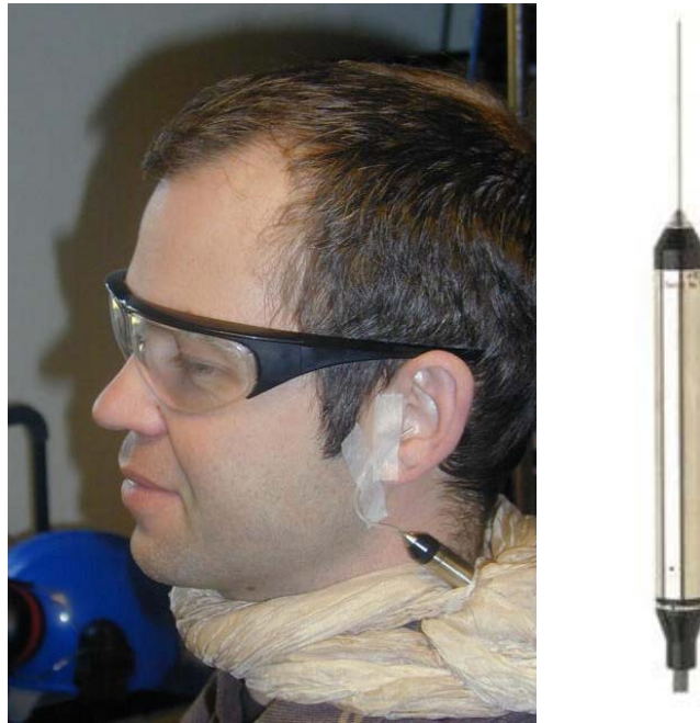
Figure 3. Left: Happy author and test person with BK 4182 probe microphone, silk scarf (borrowed from the secretary!) and spectacle no. 4. Right: The BK 4182.
