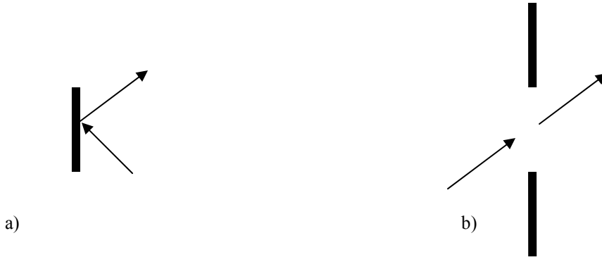
Figure 2. An example of Babinet's principle, a) reflection from a surface, b) transmission through an opening
