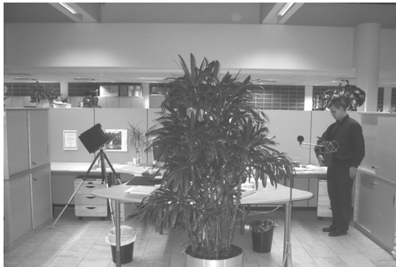
Figure 2. Measurement of RASTI between workstations. The screen is behind the palm.
