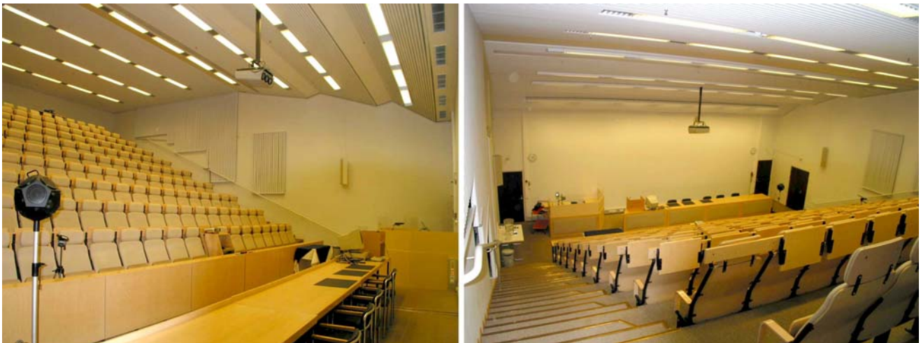
Figure 1: Auditorium views. Omnidirectional loudspeaker at location S1 and receiver at location R1 .
