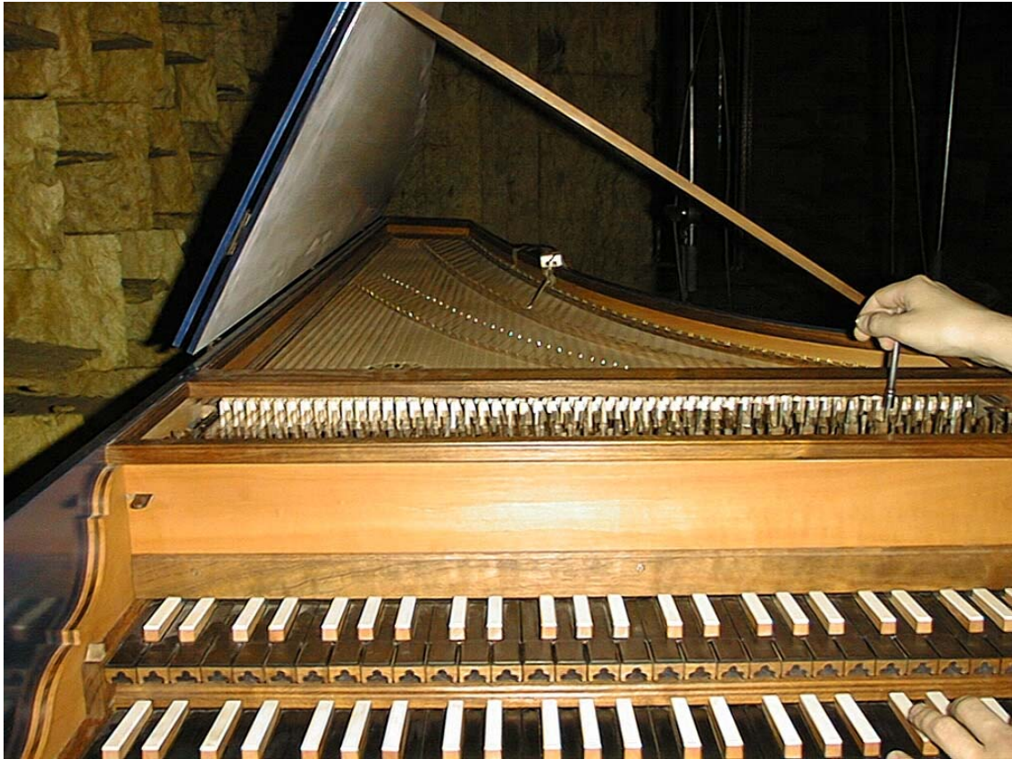
Figure 1. The harpsichord used in this study has two keyboards, three registers (string sets) and two bridges. This picture was taken during the tuning of the instrument in the large anechoic chamber of Helsinki University of Technology.
