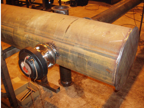
fig 3. Two loudspeakers used as input source in the test rig
