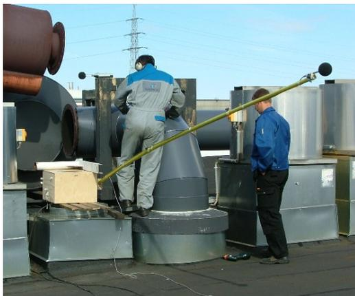
Measurement over a half hemisphere was not possible on the roof. This situation is very normal at engine manufacturers in general and causes problems to follow the classic acoustic standard. In fact only one direction could be used for significant measurements and in that direction 6 points was corrected and averaged, photo 2.
