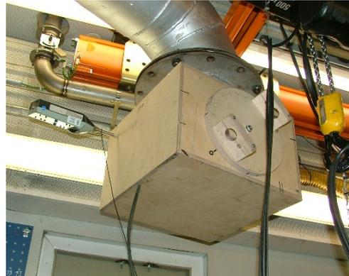
**Photo 1.** The loudspeaker box mounted for radiation into the duct. Injected sound power spectrum, first measured externally in free field and then corrected after mounting on duct.
