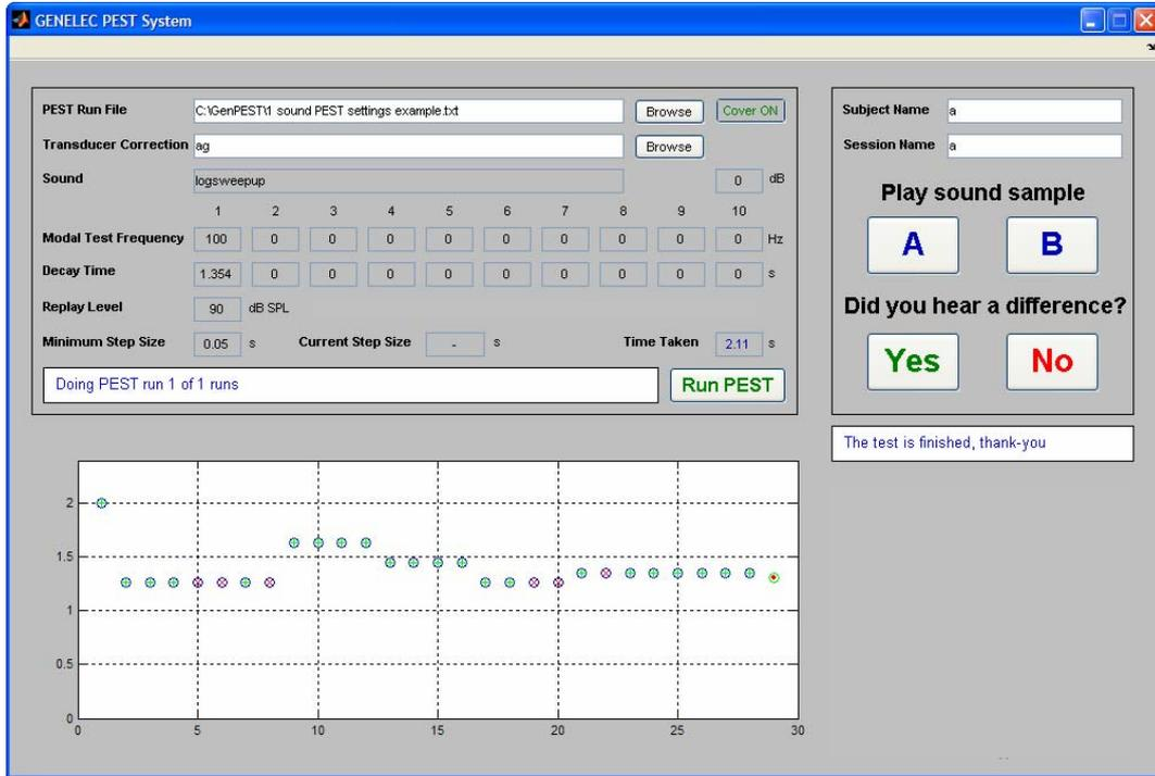
Figure 3. Listening test system graphical user interface. The left side is covered during the listening test to avoid listener bias. A  $\circ$  indicates the stimulus level being tested. A  $+$  indicates a positive response (audible difference between A & B). An  $\times$  indicates a negative response (no audible difference between A & B). The  $\odot$  indicates the result, which in this example is 1.354 s.
