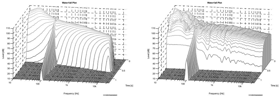
Figure 2. Left: 1/3 octave smoothed cumulative spectral decay of a 0.5 second logarithmic sine sweep (20 – 20000 Hz). It is headphone response equalized with a 1 second temporal decay at 100 Hz added. Right: The same but for 0.5 seconds of pink noise.
