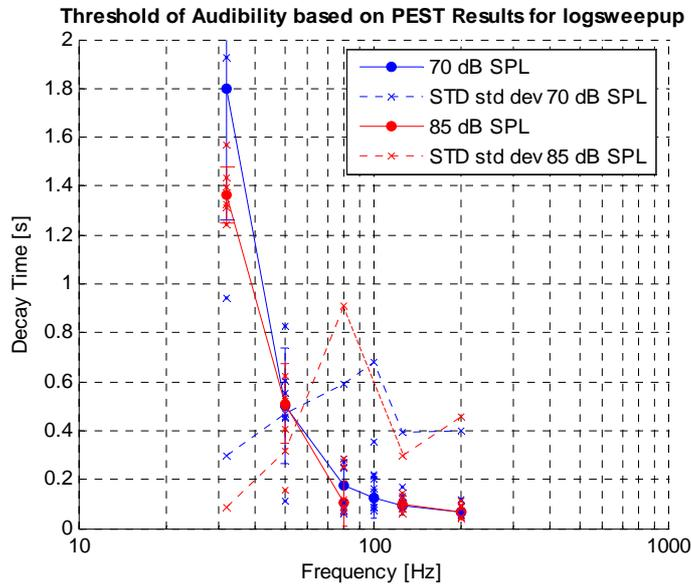
Figure 4 – Threshold of audibility at different SPL's derived from the PEST output (left) and threshold derived from a psychometric function fitted to all the listener's responses pooled together (right).
