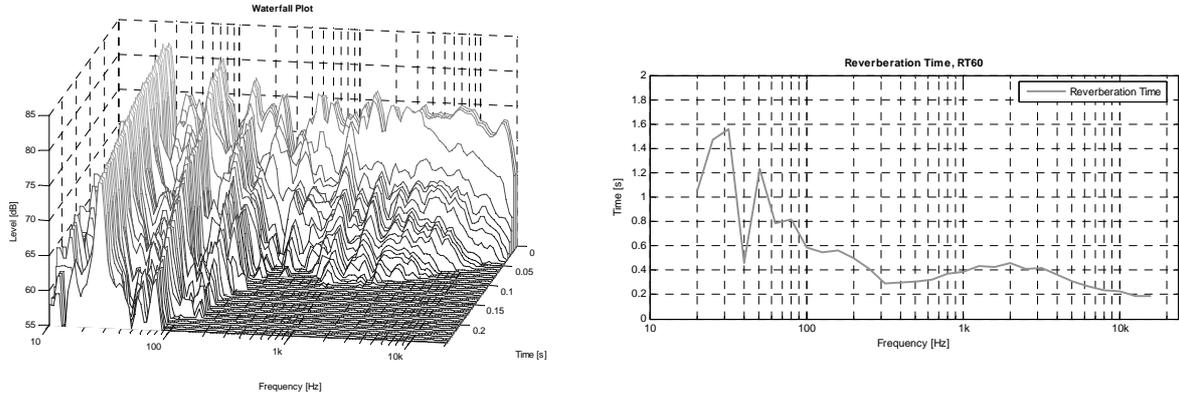
Figure 1. A measurement of a room with insufficient low frequency acoustical treatment. Left: A third-octave smoothed cumulative spectral decay showing strong room modes at 25 Hz and 75 Hz. Right: Third-octave reverberation time.
