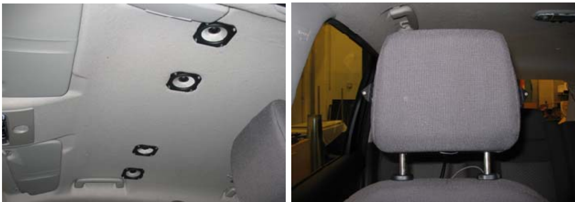
a) Loudspeakers on the roof
