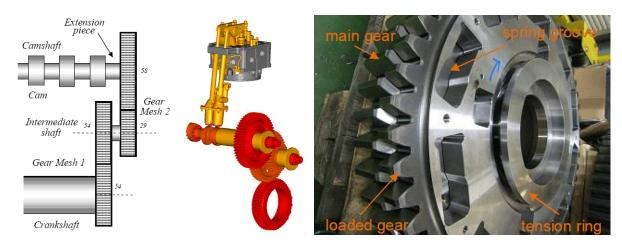
Figure 1. Left, schematic picture of the gear train system; Middle, W32 gear train model; Right, two parts of the anti-backlash large intermediate shaft gear.
