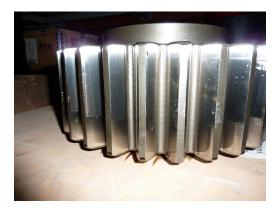
Figure 9. W6L34DF gear wheels after running for anti-backlash gear train test. Left, crank-gear; Right, small intermediate shaft gear.
