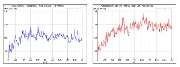
Figure 8. W6L34DF cam-gear cover inside A-weighted sound pressure level comparison, diesel 100% load, 750 rpm. Left, standard gear train; Right, anti-backlash gear train.
