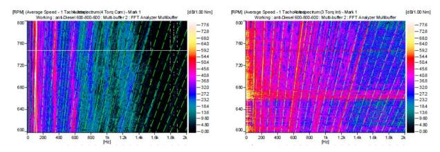
Figure 6. W6L34DF shaft torque with anti-backlash gear train application, diesel 40% load condition, 600-800-600 rpm. Left, camshaft; Right, intermediate shaft.
