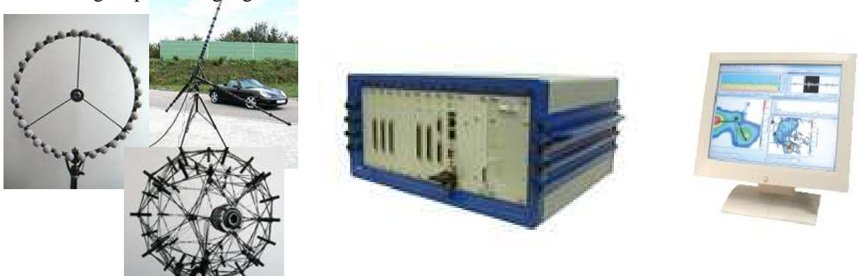
Figure 1. Typical setup up of an Acoustic Camera system: Microphone Arrays (Ring, Star and Sphere) (Left), Data Acquisition unit (Middle), Software (right)
