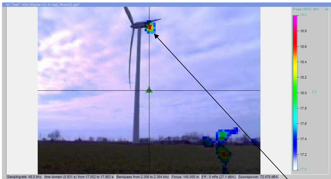
Figure 3.8: Sound Power estimation L_w=72.5 dBA from region of interest (ROI) (note: Filtered tone at 2359Hz)
