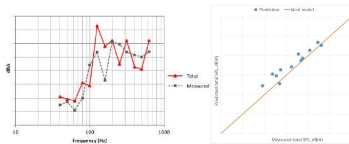
Figure 2: Validation of the model. *Left*: Measured vs simulated SPL spectrum in an elevator car. *Right*: Measured vs predicted total SPL level in several different elevators.
