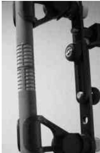
Figure 2. *Mounting of 2 Schoeps MK4Vg capsules (with CMC5 bodies) above one another to achieve perfect time alignment for horizontal pickup.*
