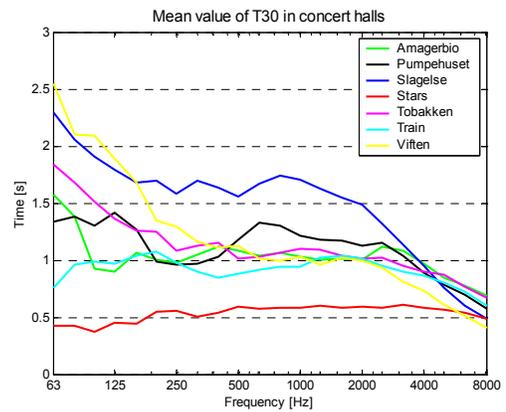
Figure 2. Position averaged T30 per 1/3 octave in all halls. NB: Tobakken and Viften were measured with PA.
