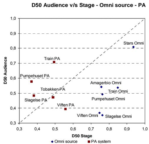
Figure 4. D50 (63-250 Hz) for audience and stage area measured with PA and omni source.
