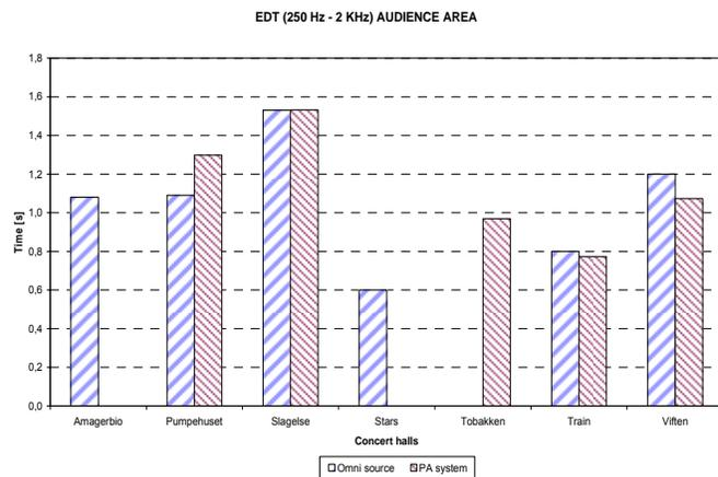
Figure 1. EDT comparison when measured with PA and omni source in the range of 250 Hz – 2 KHz.
