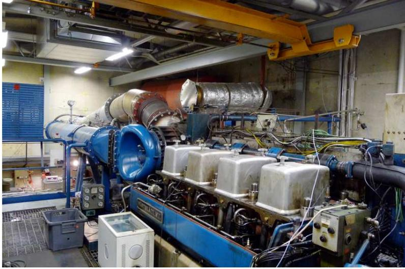
Figure 1: The test engine, Wärtsilä Vasa 4R32 in VTT engine laboratory.
