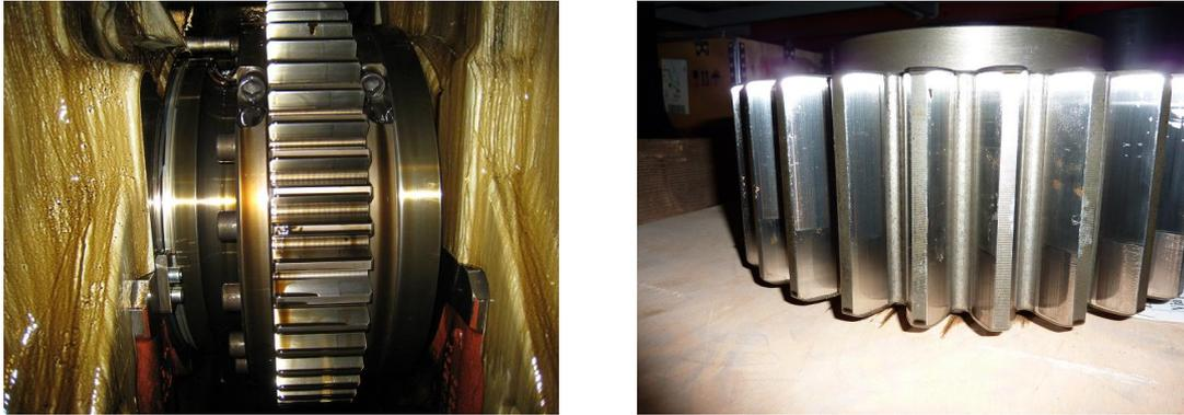
Figure 9. W6L34DF gear wheels after running for anti-backlash gear train test. Left, crank-gear; Right, small intermediate shaft gear.
