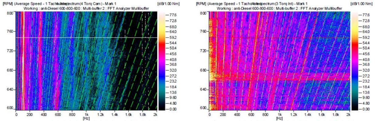
Figure 6. W6L34DF shaft torque with anti-backlash gear train application, diesel 40% load condition, 600-800-600 rpm. Left, camshaft; Right, intermediate shaft.
